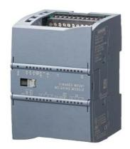
SIMATIC S7-1200 or Stand Alone, SIWAREX WP241, single-channel weighing module for conveyor belt scales and solids flowmeter with analog load cells / strain gauges (full bridges), 4xDI, 4xDQ, 1xAQ, 1xRS485, 1xEthernet, 1xLC load cell interface (1-4mV/V), Detailed load cell diagnostics with digital junction box SIWAREX DB (7MH5001-0AD20 or 7MH5001-0AD01)
