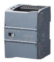
SIMATIC S7-1200 or Stand Alone, SIWAREX WP231, single-channel legal-for-trade weighing module for platform or hopper scales with analog load cells / strain gauges (full bridges), 4xDl, 4xDQ, 1xAQ, 1xRS485, 1xEthernet, 1xLC load cell interface (1-4mV/V)), attention: for legal-for-trade applications please follow the local laws applying in the country of verification! Detailed load cell diagnostics with digital junction box SIWAREX DB (7MH5001-0AD20 or 7MH5001-0AD01)
