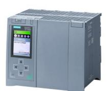
SIMATIC S7-1500T, CPU 1517T-3 PN/DP, Central processing unit with work memory 3 MB for program and 8 MB for data, 1st interface: PROFINET IRT with 2port switch, 2nd interface, Ethernet, 3rd interface, PROFIBUS, 2 ns bit performance, SIMATIC Memory Card required
