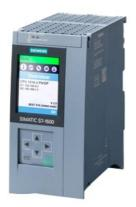
\*\*\* spare part \*\*\* SIMATIC S7-1500, CPU 1516-3 PN/DP, central processing unit with work memory 1 MB for program and 5 MB for data, 1st interface: PROFINET IRT with 2-port switch, 2nd interface: PROFINET RT, 3rd interface: PROFIBUS, 10 ns bit performance, SIMATIC Memory Card required
