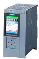
\*\*\* spare part \*\*\* SIMATIC S7-1500F, CPU 1515F-2 PN, central processing unit with work memory 750 KB for program and 3 MB for data, 1st interface: PROFINET IRT with 2-port switch, 2nd interface: PROFINET RT, 30 ns bit performance, SIMATIC Memory Card required
