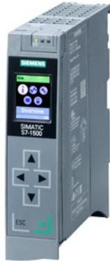
SIMATIC S7-1500T, CPU 1511T-1 PN, Central processing unit with Work memory 225 KB for program and 1 MB for data, 1st interface: PROFINET IRT with 2-port switch, 60 ns bit performance, SIMATIC Memory Card required
