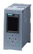
\*\*\*spare part\*\*\* SIPLUS S7-1500 CPU 1515R-2 PN TX rail based on 6ES7515-2RM00-0AB0 with conformal coating, -40...+70 °C, OT4 with ST1/2 (+85 °C for 10 minutes), heat sink, no PU usable, central processing unit without display with work memory 500 KB for program and 3 MB for data, 1st interface: PROFINET with 2-port switch, 2nd interface: PROFINET RT, SIMATIC Memory Card required
