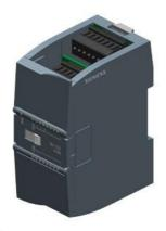
SIPLUS S7-1200 SM 1234 4AI/2AQ rail based on 6ES7234-4HE32-0XB0 with conformal coating, -25...+60 °C, OT1 with ST1/2 (+70 °C für 10 minutes), SM 1234, 4 AI/2 AQ, +/-10 V, 14-bit resolution or 0 (4)-20 mA, 13-bit resolution
