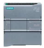
SIPLUS S7-1200 CPU 1212C DC/DC/DC T1 rail based on 6ES7212-1AE40-0XB0 with conformal coating, -25...+60 °C, OT1 with ST1/2 (+70 °C für 10 minutes), compact CPU, DC/DC/DC, onboard I/O: 8 DI 24 V DC 6 DQ 24 V DC 2 AI 0-10 V DC, power supply: 20.4-28.8 V DC program/data memory 50 KB
