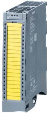
SIPLUS S7-1500 F-DQ 8x24VDC/2A based on 6ES7526-2BF00-0AB0 with conformal coating, -30...+60 °C, F digital output module, 35 mm overall width; up to PL E (ISO 13849-1)/ SIL3 (IEC 61508)
