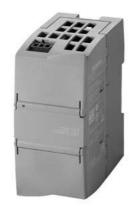
SIPLUS NET CSM 1277 based on 6GK7277-1AA10-0AA0 with conformal coating, 0...+60 °C, Compact Switch Module CSM 1277 connection SIMATIC S7-1200 and up to 3 further nodes to Industrial Ethernet with 10/100 Mbps
