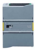
SIPLUS S7-1200 SM 1226 F-DI 16x24VDC based on 6ES7226-6BA32-0XB0 with conformal coating, -25...+55  $^{\circ}$ C, F-DI 16x 24 V DC, PROFIsafe, 70 mm width, up to PL e (ISO 13849-1)/ SIL3 (IEC 61508)
