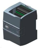
SIPLUS S7-1200 SM 1223 16DI/16DQ RLY based on 6ES7223-1PL32-0XB0 with conformal coating, -40...+70 °C, start up -25 °C, digital input/output 16 DI/16 DQ, 16 DI 24 V DC, sink/source, 16 DQ, relay 2 A
