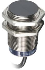
Inductive proximity sensors XS, inductive sensor XS6 M30, L62mm, brass, Sn15mm, 12...48 VDC, cable 2 m
